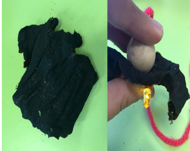
Image 2. On the left a coffee ground bioplastic and on the right a lamp created with it
